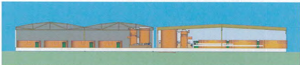
Figure 9. Profile View Rendering of the Freshwater Tissue Pulp Mill Warehouses with Recirculating Aquaculture Systems to produce 500,000 kg of fish per year.
