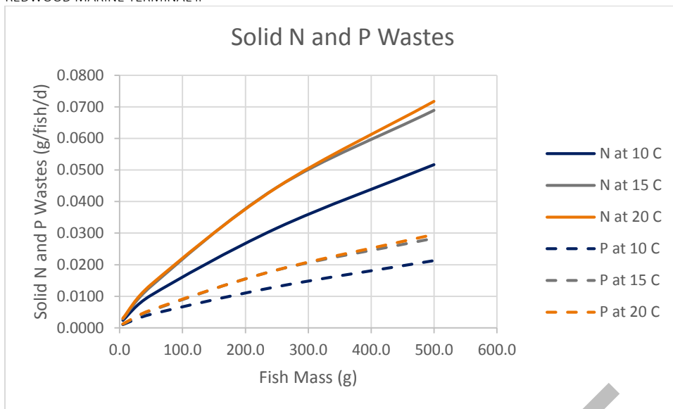
Figure 3. Estimated daily production of solid N and P wastes by individual steelhead trout
